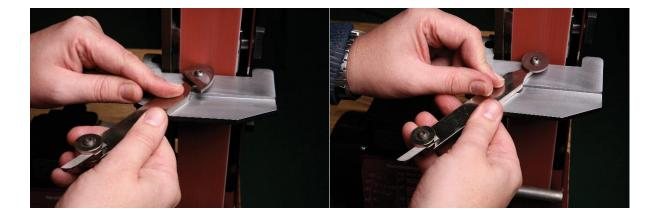
The end with the clamp is used to sharpen the RS211C and RS212C cutters (see picture below). Clamp the cutter in the holder with the flat top of the cutter facing up. Set the table to 80 degrees and place the holder flat on the table and sharpen the tip.
